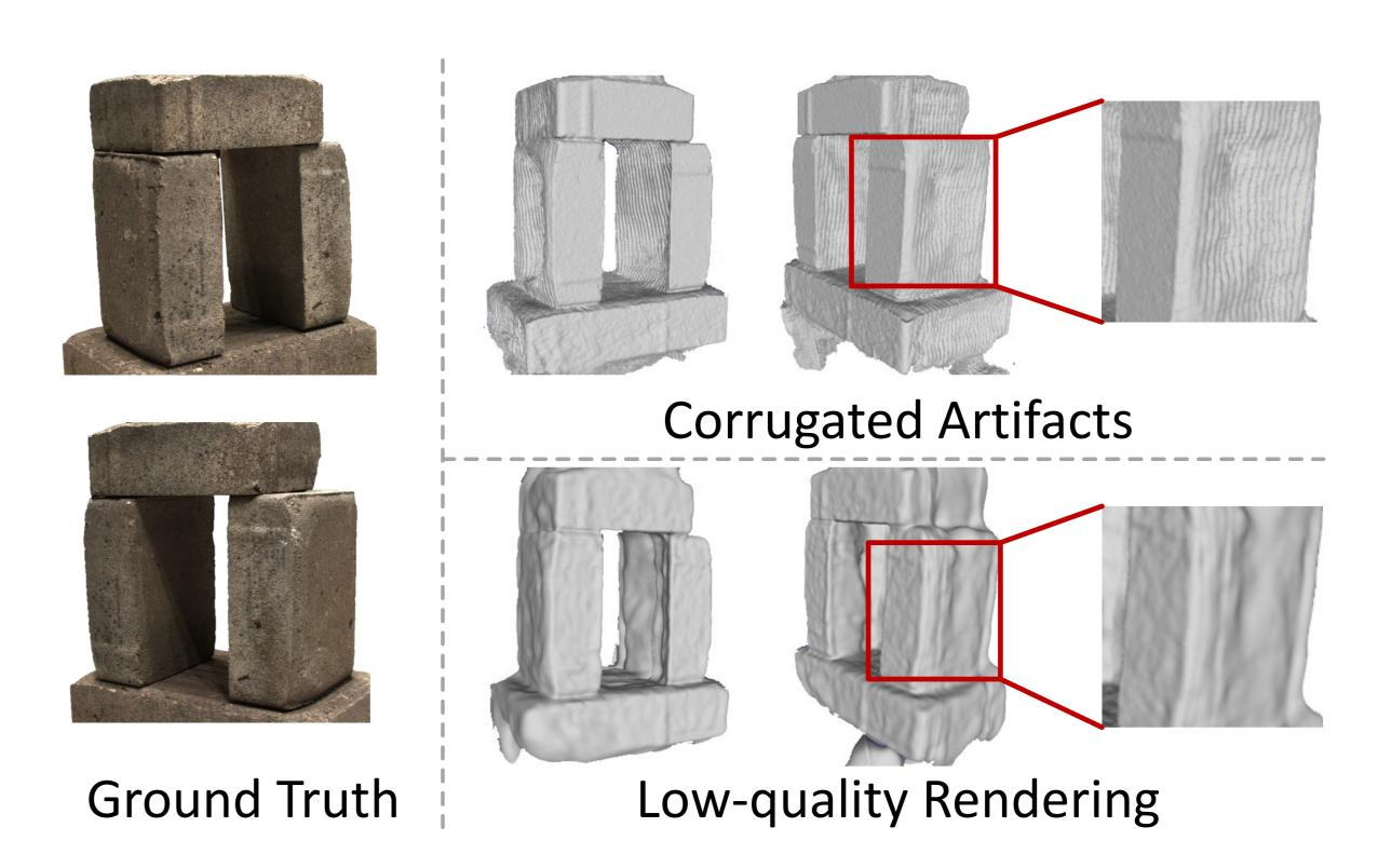
To improve view quality and reduce artifacts, we replace positional encoding with a **mixed Sinus-ReLU activation**, using sinus for the encoder and ReLU for the decoders.
