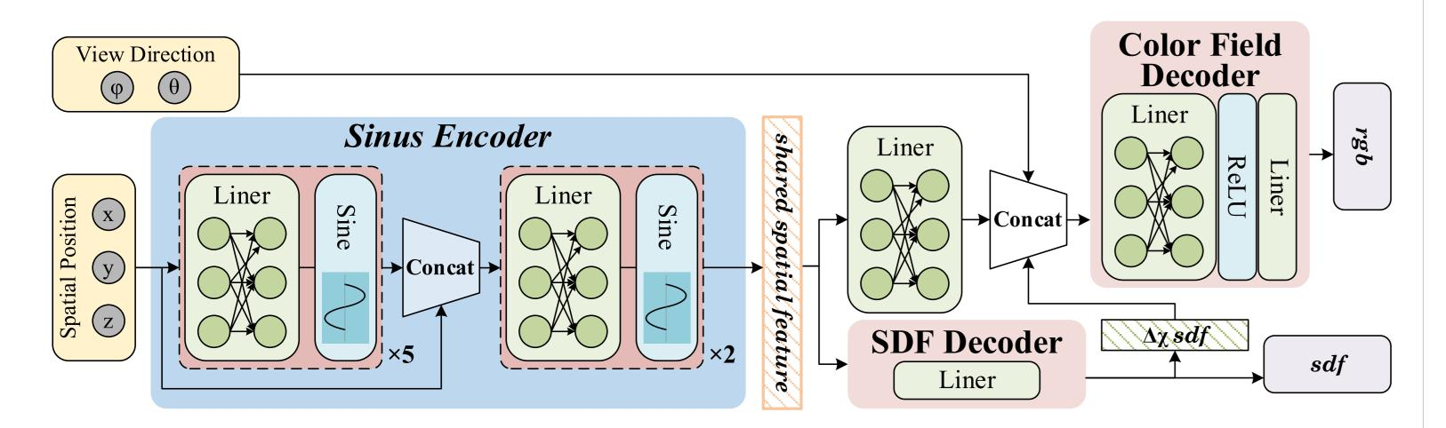
Compared to the common paradigm, where the color field is conditioned on  $[x, v, \nabla_x sdf, F_{sdf}]$ , we allow the SDF and color field to share the **same feature** F from the encoder, while obtaining the spatial position through an additional forward pass.
